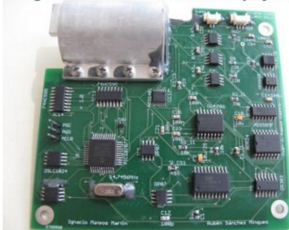
Flight model of the CubeSat payload
