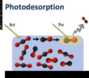
Molecules in the surface receiving **photon energy** to break intermolecular forces and desorb
