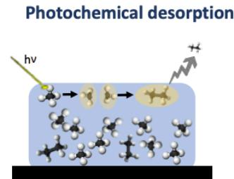
Molecules formed in the surface releasing **their formation energy** to break intermolecular forces and desorb
