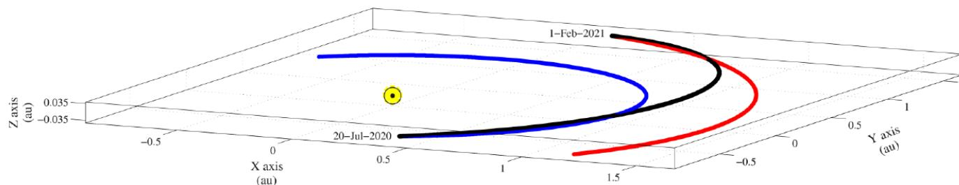
Figure 4: Optimal transfer orbit from Earth to Mars from 20th July 2020 to 1st February 2021.
