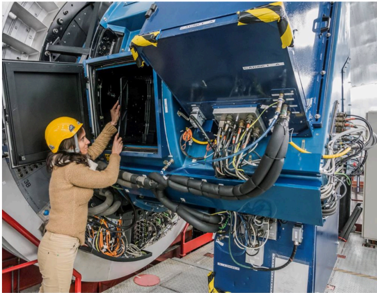
Left: OSIRIS mask exchanged operation as being done by a GTC staff member. Right: Mock-up image of the MAAT module inserted in the OSIRIS Cassette structure (Credit: GTC).
