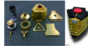
#AthenaNuggets 43: First development model of the X-IFU Focal Plane Assembly ready for test
