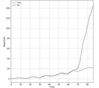
Red dashed lines denote the linear analytic results whereas blue dashed lines denote the numerical results. • The increase of both physical quantities with time, predicted by linear theory, is owing to phase-mixing alone. The dramatic increase towards the end of the full nonlinear simulation is due to the triggering of the Kelvin-Helmholtz instability.
