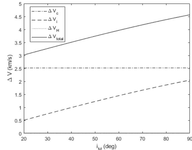
Figure 3: Manoeuvres impulse needed to achieve the areostationary orbit.
