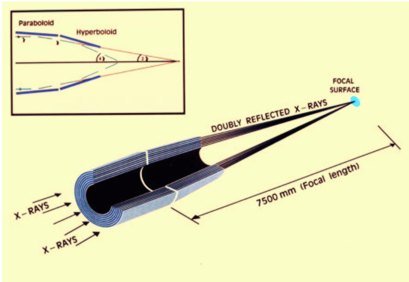
Fig. 1.: Scheme of the grazing incidence optics on the *XMM-Newton* X-ray telescopes (from ESA)
