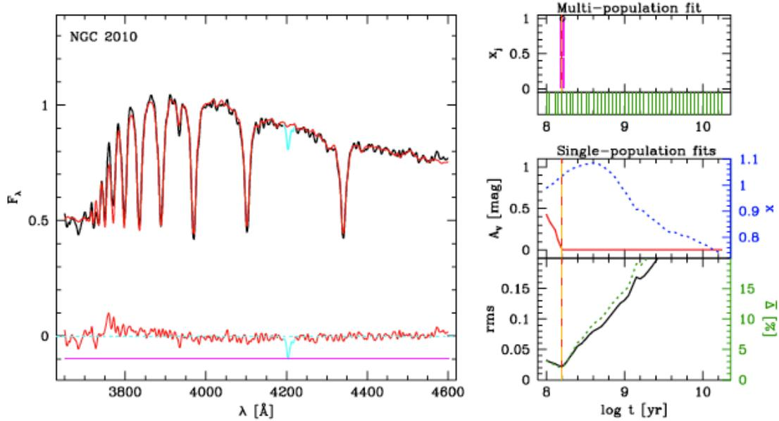
Figure 4: Starlight results for the LMC stellar cluster NGC 2210. Models are from [66]. Observed (black), best-fit (red) spectra and residual (bottom) are plotted on the left. Results of the multi-SSP fit is on the right. *Middle right*: Best fit  $A_V$  and  $x$  for single-SSP fits as a function of age. Solid (red) and dashed (orange) vertical lines mark the best single-SSP age and mean age in the multi-SSP fit. *Bottom right*: rms and  $\bar{\Delta}$  figures of merit as a function of age.
