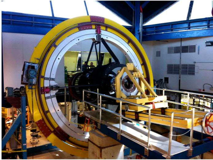
Figure 3: Telescope simulator at Fermilab. The purpose of this setup is to mechanically test the fully integrated camera, filter and shutter jukebox and hexapod adjusters. Lenses are directly shipped to the telescope, so mock weights are used instead. Also the cryogenic system and the detector grounding are tested with this fixture.
