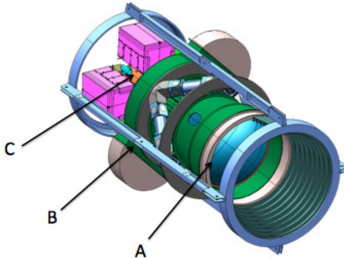
Figure 1: Diagram of DECam, showing the positions of the optical corrector (A), shutter and filter system (B) and camera vessel (C).
