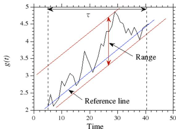
Figure 1: This shows how the Rescaled Range Analysis works. In the example instead of correcting the series by the mean, a reference line is chosen and the differences of the maximum and the minimum are calculated from it for each timescale.
