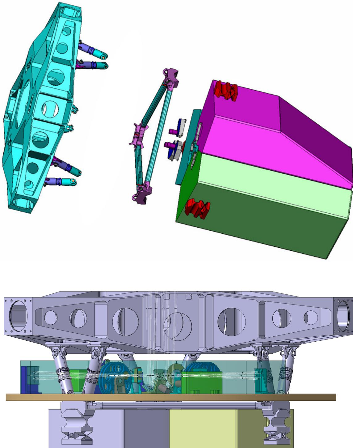
Figure 1: *Top:* Mounting of HIRDES and LSS on the optical bench. *Bottom:* Mounting of ISIS on the OB.
