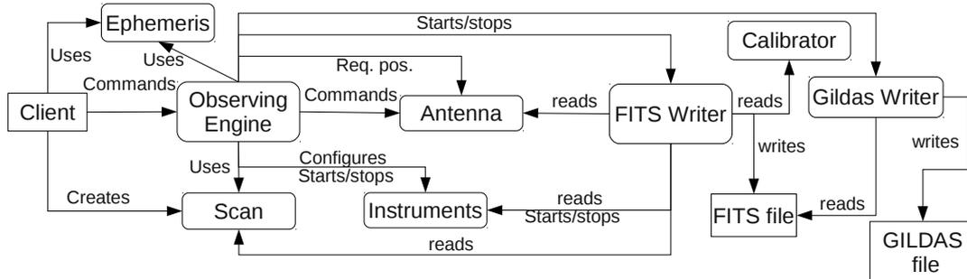
Figure 1: Relationship between the components during a single dish observation.
