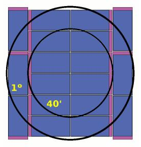
Figure 1: Distribution of the CCDs in the PAUCam instrument, optimized for a 60 arcmin field of view and the chosen detectors.
