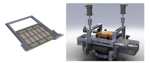
Figure 3: *Left*: One filter tray with the holders to install each narrow and broad band filter. *Right*: Filter tray interchange system with sixteen trays.
