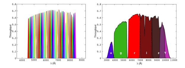
Figure 2: Theorical throughput for the forty narrow-band filters (*left*) and for the six broadband filters (*right*). These are calculated with models of the atmosphere, telescope and filter transmision and the quantum efficiency of HPKK detectors.
