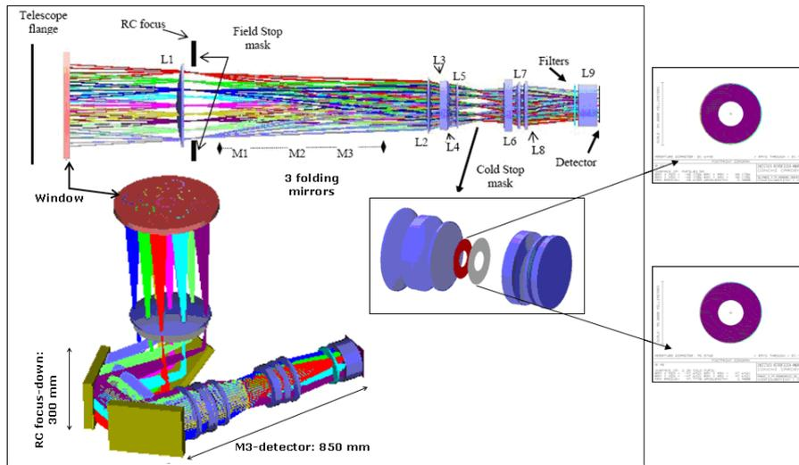
Figure 2: PANIC optics layout, including the unfolded layout.
