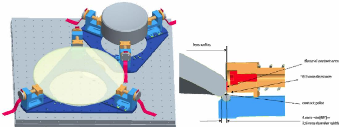
Figure 9: *Left*: set-up for the PANIC lenses cryogenic tests acceptance. *Right*: a detail of the mechanical low-stress mounting.
