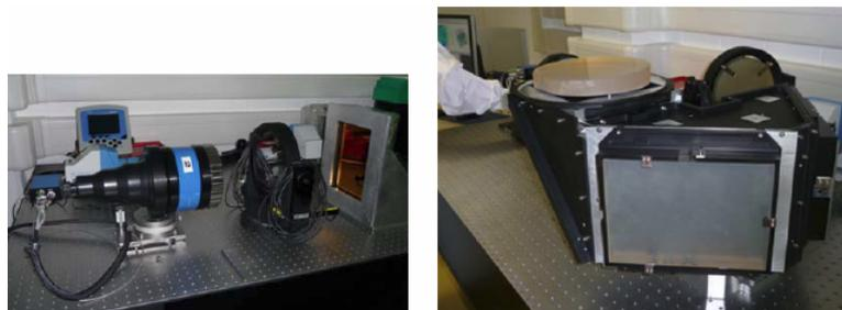
Figure 8: *Left*: doing an interferogram of one PANIC mirror. *Right*: Mirror structure integrated and aligned.
