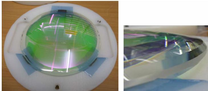
Figure 7: L8 in its packaging from manufacturing. *Right*: a detail showing the chambers of the lens.
