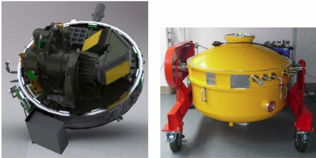
Figure 5: *Left:* The layout of PANIC with cryostat open and turned upside down (left). Light enters from below, is folded by 3 mirrors (to the upper left) parallel to the optical bench, passes cold stop and filter wheels and is focused on the detectors. *Right:* real PANIC cryostat with its lab's caddy at the laboratory. PANIC optics layout, including the unfolded layout.
