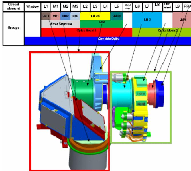
Figure 6: The grouping of the mechanics corresponding to optical groups.
