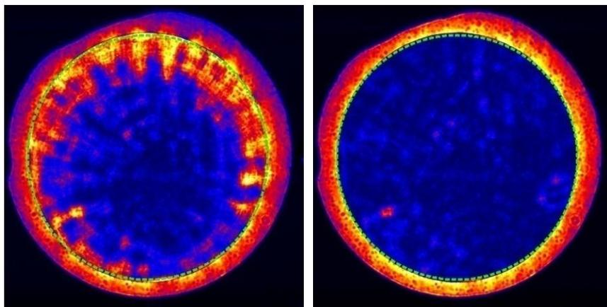
Figure 3: Focusing the starlight onto the vortex mask (*right*) instead of onto the detector plane (*left*) has led to significant darkening of the Lyot pupil plane, and so to much better rejection of starlight.
