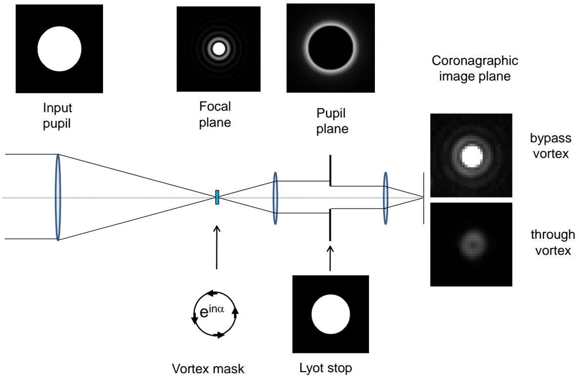
Figure 2: Layout and operation of the vortex coronagraph. Note that in the post-vortex Lyot plane, all of the starlight lies outside of the original pupil, and so can be easily rejected.
