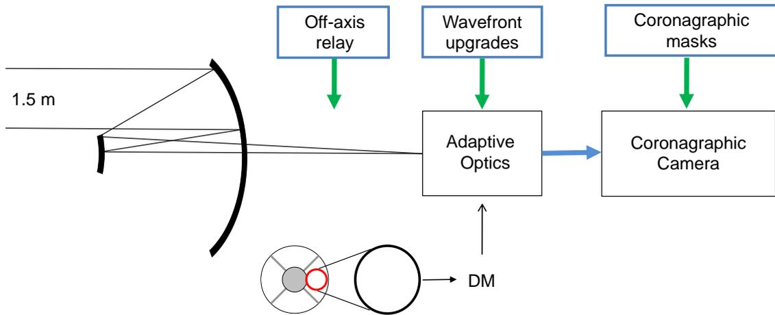
Figure 1: Layout of the Palomar Well-Corrected Subaperture. The resultant optical system is that of a coronagraphic 1.5 m off-axis telescope.
