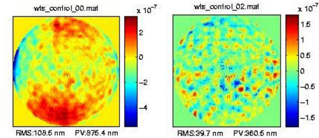
Figure 4: Non-common path speckle reduction by means of phase retrieval [3] has led to improvement in wavefront quality from (*left*)  $\approx 110$  nm rms to (*right*)  $\approx 30$ -40 nm rms.
