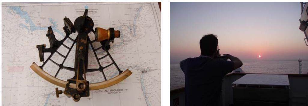
Figure 2: *Left*: Modern sextant for teaching astronomical navigation, in use at La Coruña University. *Right*: Measuring the solar azimuth with an alidade.
