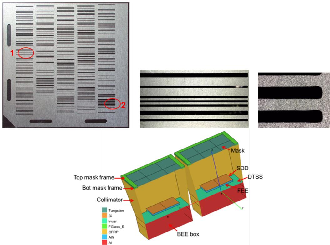
Figure 5: Left: View of the manufacturing of  $\frac{1}{4}$  size of the coded mask. Centre: Zoom 1 shows a group of slits in a column. Zoom 2 illustrates the detail of the slit chamfer. Right: WFM camera thermal model
