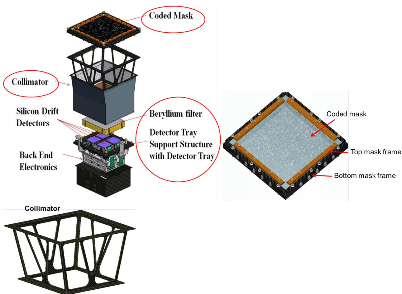
Figure 3: Left: Exploded view of the WFM camera elements. Centre: Coded mask assembly. Right: Collimator structure
