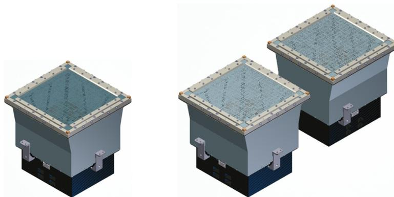
Figure 2: Left: One camera providing “1.5D” positions. Right: One camera pair results from the combination of two orthogonal cameras; it provides accurate 2D positions
