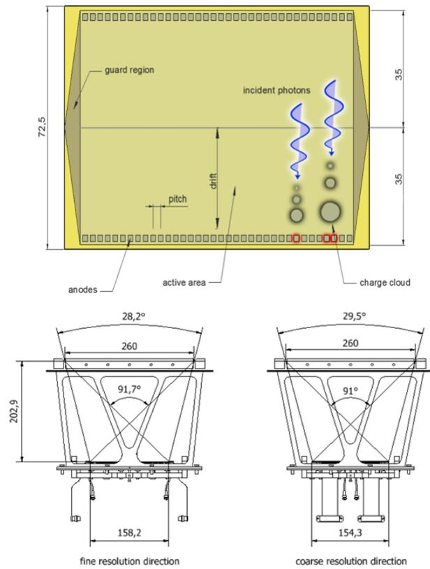
Figure 1: Left: Working principle of the SDD detector and dimensions, in mm, of the SDD tile. Right: Optical configuration of a WFM camera showing the fine and coarse resolution
