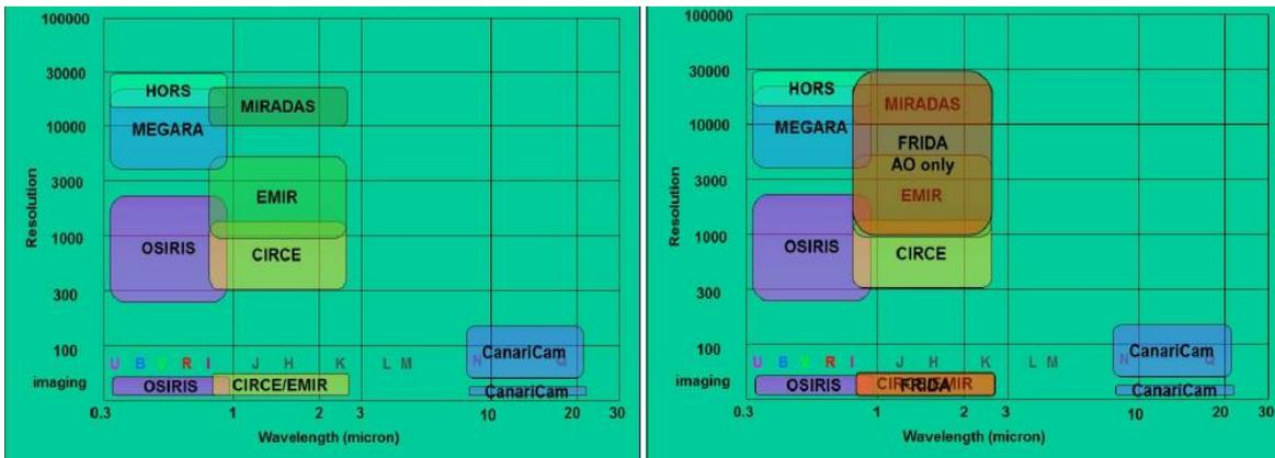
Figure 4: Global scheme of the GTC instrumentation available by 2019-2020.
