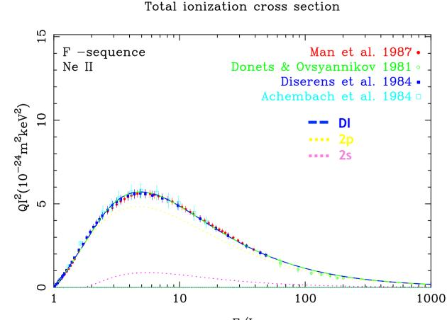
**DI data fitting example**.<sup>E</sup><sup>/</sup>Ne II for F isoelectronic sequence. Colored dots are the different datasets showed in the figure. Dotted pink line is 2s subshell, dotted orange line 2s subshell, dashed blue line DI contribution.
