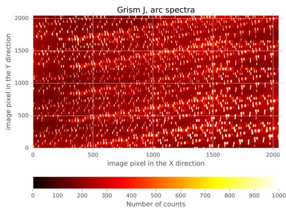
Arc lamp exposure obtained with EMIR in the J band, showing  $\sim 53$  spectra. The EMIR Configurable Slit Unit is responsible for the multi-slit pattern in the instrumental focal plane. The X axis corresponds to the spectral direction whereas the Y axis is the spatial direction.
