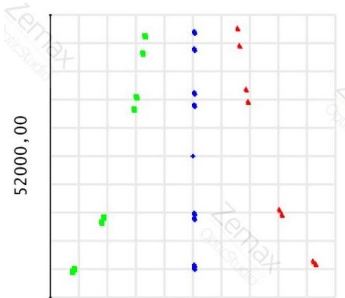
Figure 3: Matrix spot diagram.
