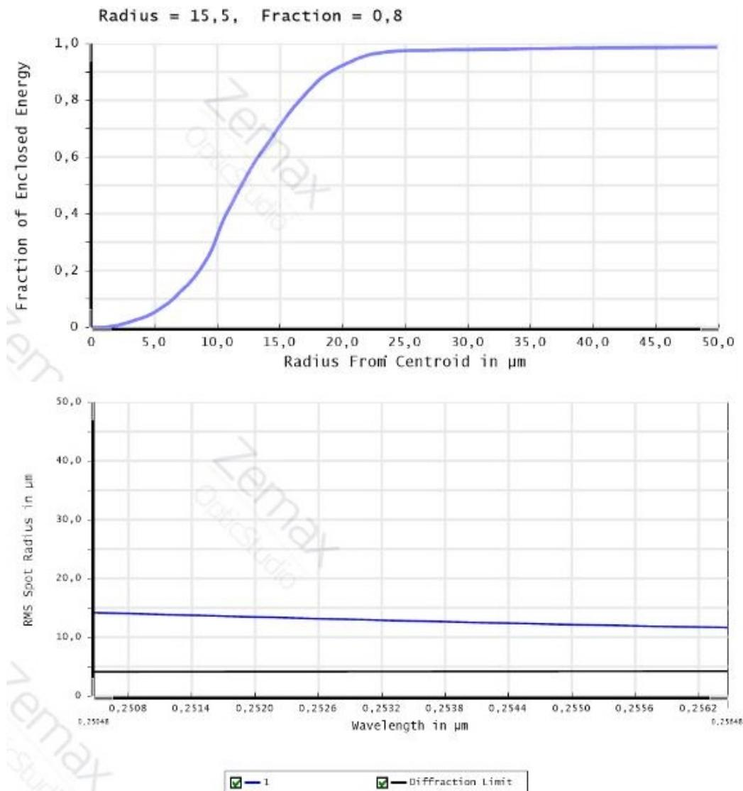
Figure 5: Encircled energy and RMS spot radius for  $m = 26$  in 254 nm.
