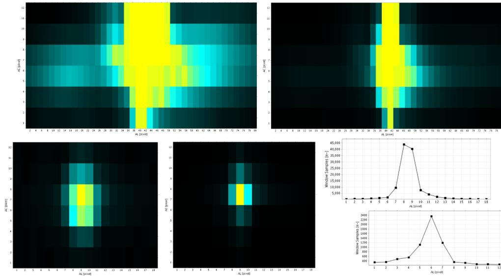
Figure 3: Astrometric 2D and 1D observation window examples. Total window flux decreases from top-left to right-bottom pane.
