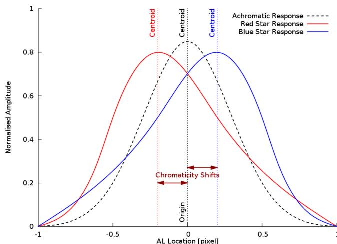
Figure 4: Definition of LSF origin with respect the image geometric centroid adopted for chromatic shift correction
