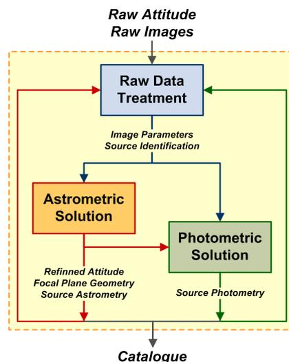
Figure 2: Main processing chains and interdependencies; from spacecraft raw data to the source catalogue parameters.
