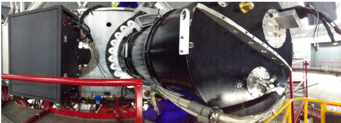
Figure 4: The CIRCE NIR instrument attached to the elevation ring in one of the GTC Folded Cassegrain stations.
