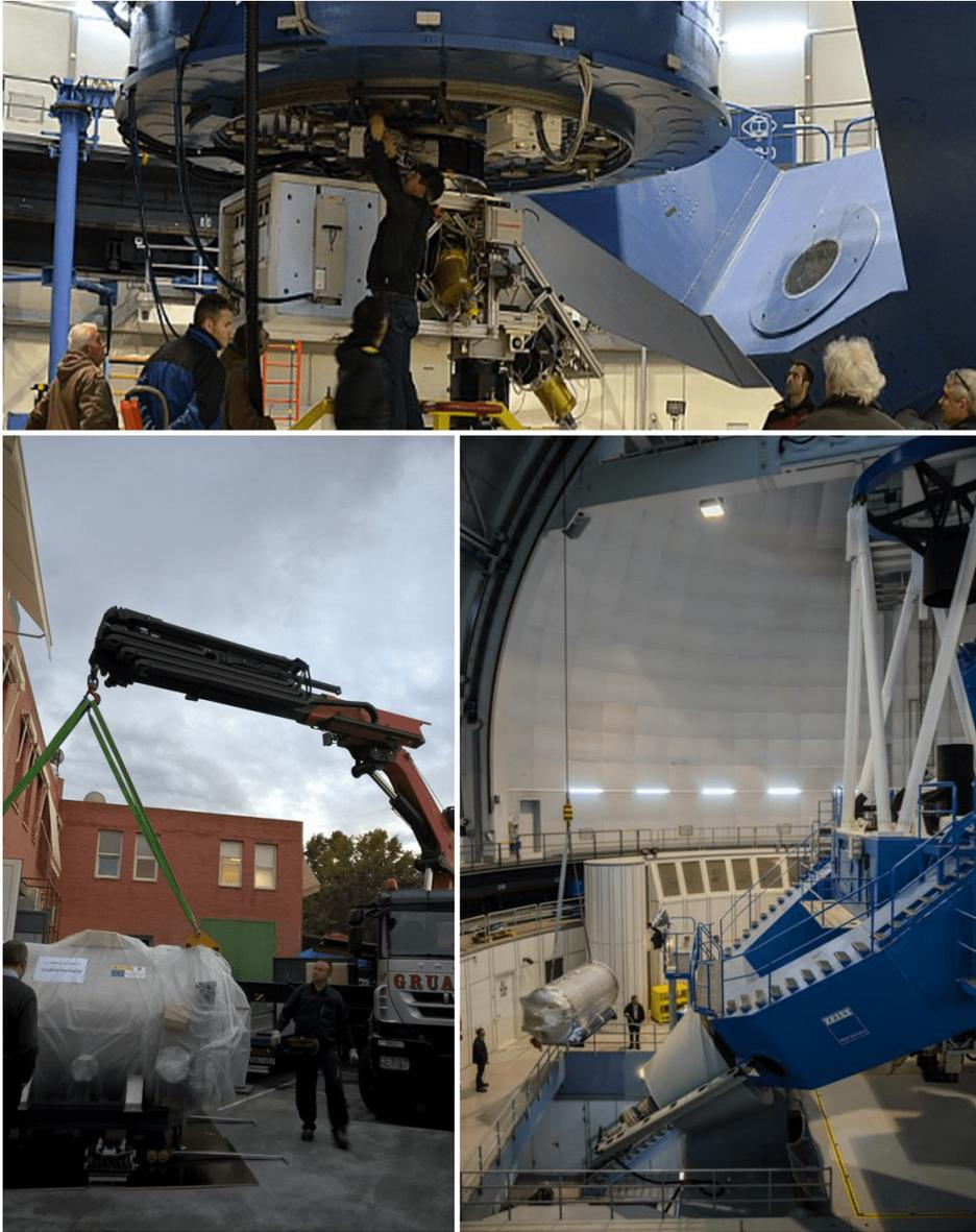
Figure 3: From top to bottom, a few more details on the transport (top) final location of the channel inside its climatic temperature-stabilised room (middle) and some of the subsystems (not all of those showed here traveled inside the spectrograph during the transport) of the NIR spectrograph (bottom).
