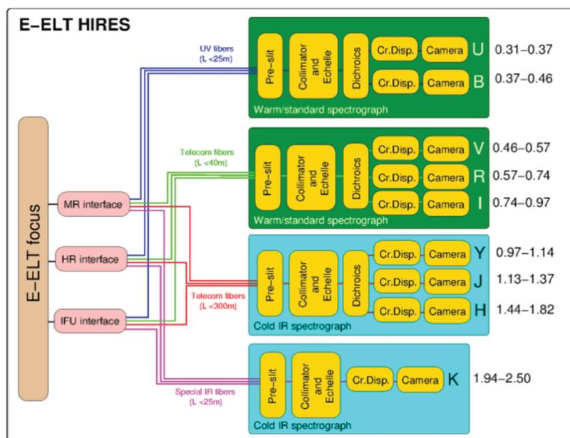
Figure 7: Possible HIRES architecture with wavelength splitting in four spectrographs. Wavelength splitting is indicated only for illustrative purposes and will be the results of the trade-o analysis conducted during the Phase A study.
