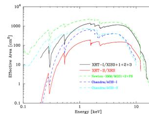
**Effective area vs Energy [10].** The figure shows a comparison of the effective area of the main X-ray satellites. The performance of *Suzaku* XIS (in black) are comparable with XMM-Newton EPIC (in green). Since 2006, XIS 2 was no available, therefore the  $A_{eff}$  was a bit lower.
