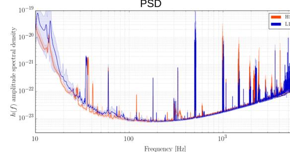
Noise budget of the Advanced LIGO detector. In order to detect the GW signal a denoising of the data is performed.
