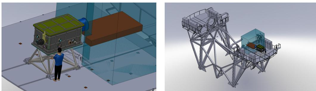
Figure 5: Rendered images of FRIDA at the Nasmyth platform showing the envelope of GTCAO.
