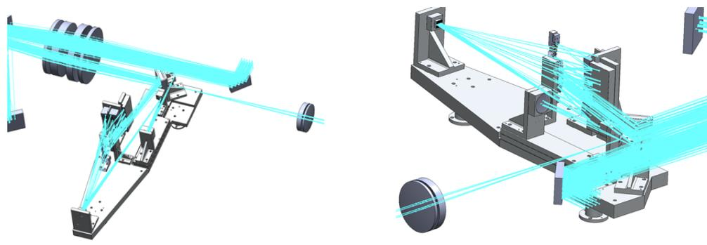
Figure 4: A rendered image of the IFU and the spectrographs optics, with ray tracing indicated.
