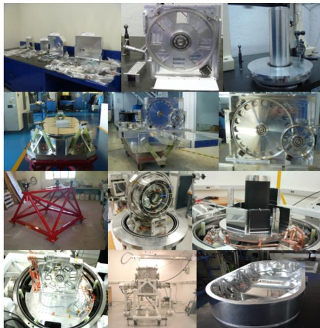
Figure 8: Examples of mechanical pieces fabricated by CIDESI. The image shows filter holders, the focal plane wheel and pupil wheels, the grating carousel, the support structure, the collimator and FP wheel during cold tests, one of the large test dewars, FCTF, and the LN2 container of FRIDA
