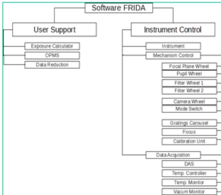
Figure 9: Tasks related to the high level software control and data acquisition of FRIDA
