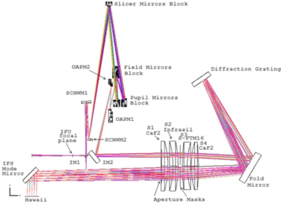
Figure 3: Optical lay-out of the integrak field unit and the spectrograph.
