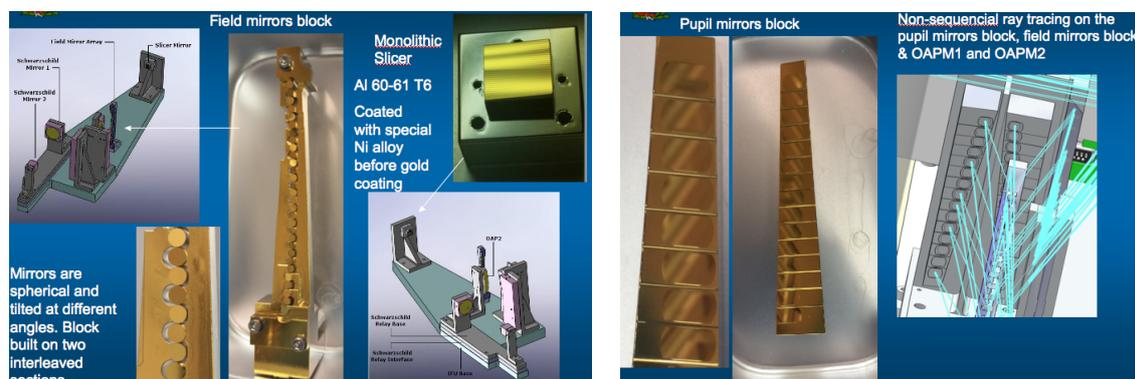
Figure 7: The finished and coated monolithic slicer, field mirrors block and pupil mirrors block are shown next to graphics that identify their location in the integral field unit.
