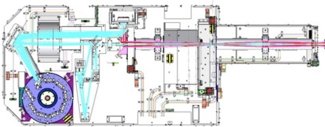
Figure 1: The optical bench lay-out of FRIDA. The red beam tracks the path in imaging mode and the cyan beam shows the path in IFS mode. The beam enters from the right.
