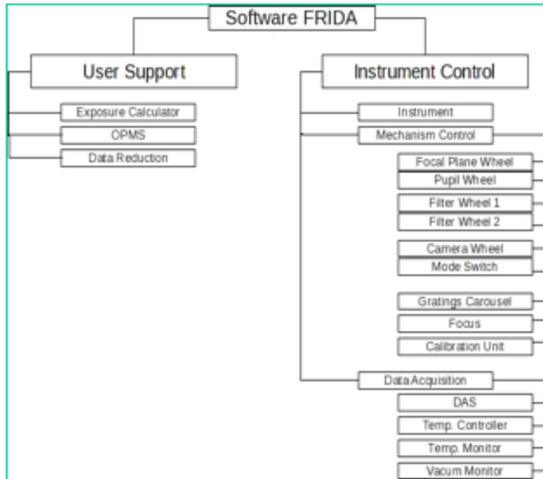
Figure 9: Tasks related to the high level software control and data acquisition of FRIDA
