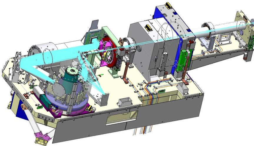
Figure 2: A rendered image of FRIDA with the beam path of the IFS mode indicated in cyan. The beam enters from the right.
