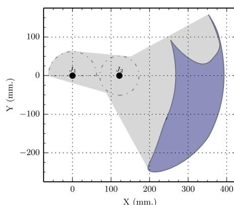
Some tip positions can be reached by two configurations (different  $J_4$  pos.) as can be appreciated in the 3D workspace.
