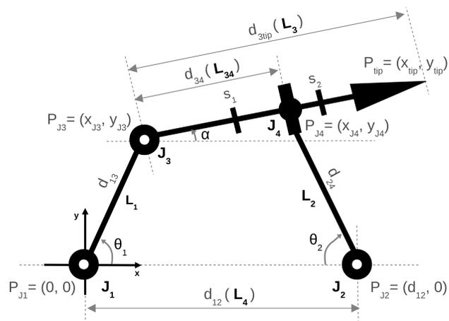
Figure 2: The arm model is a close-loop kinematic chain. Joint  $J_4$  must be always between stop positions  $s_1$  and  $s_2$ . The 2 DoF of the mechanism are represented by  $\theta_1$  and  $\theta_2$ , where  $\theta_1 \in [0, \pi]$  and  $\theta_2 \in [0, 2\pi]$ .
