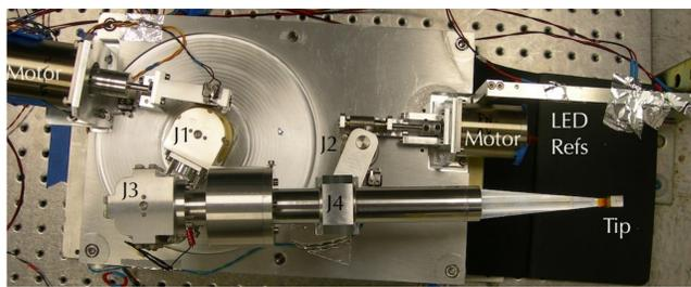
Figure 1: The full-scale MXS probe prototype P2a shown from an aerial view.
