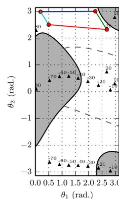
Figure 4: A SoP in articular space that satisfies motor controller constraints.
