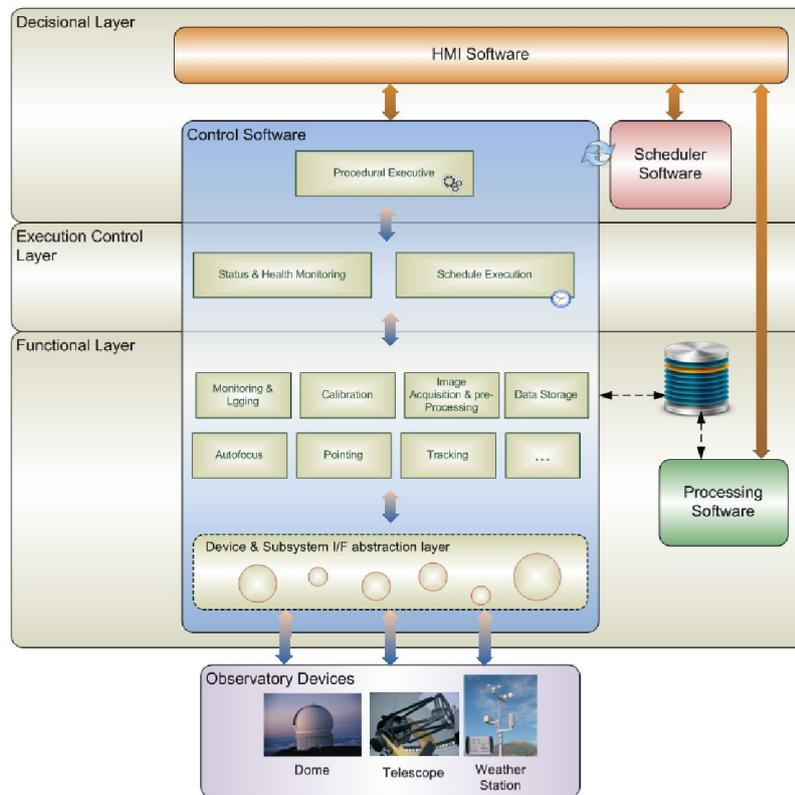
Figure 1: Software high-level architecture.
