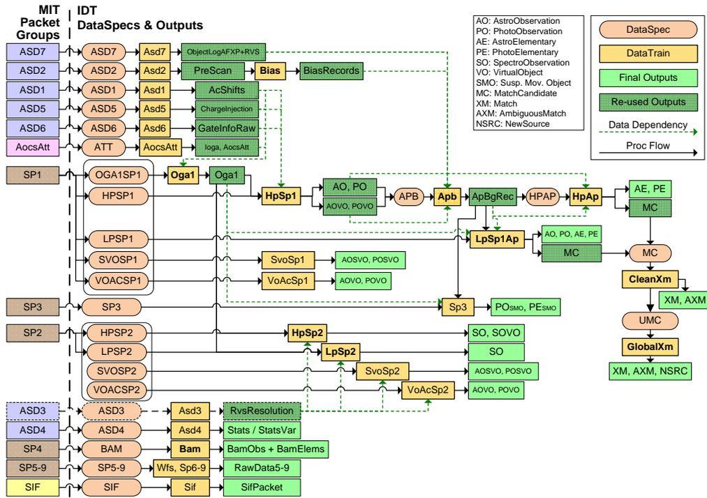
Figure 2: Overview of IDT, with its main processing modules (or Data Trains), flow control elements (or Data Specs), inputs (MIT Packet Groups), outputs and dependencies.
