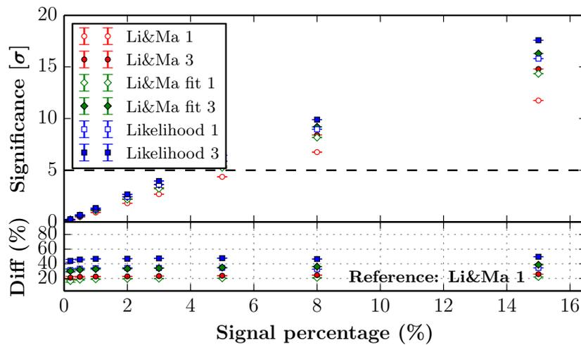
Figure 4: Significance of different methods for Monte Carlo simulations. For each method, we test the ‘1 OFF region’ and the ‘3 OFF region’ cases. The  $5\sigma$  limit (the usual detection threshold) is drawn as an horizontal dashed line.
