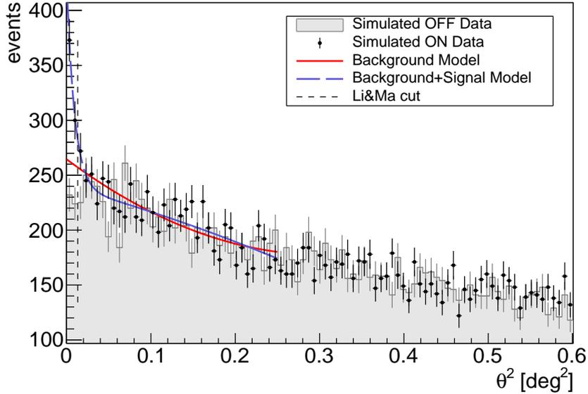
Figure 2: Testing the method with simulated samples for an ON region with 8% excess events (black points) and a single OFF region (shaded region). Background-only model (red line) and background+signal model (green line) are shown as reference. The dashed vertical line shows the region used by the *Li&Ma* method.
