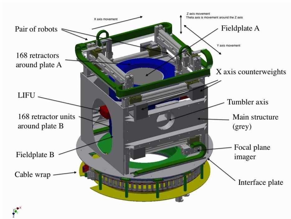
Figure 2: The final design of the WEAVE fibre positioner. Light from the primary mirror enters from below. Of the two field plates, plate A is shown in the configuration position and plate B (below) is in the observing position. A 180-degree rotation around the tumbler axis reverses their positions, while a 90-degree rotation places the large IFU (LIFU, red in the image) in the observing position. The two x-y robots are at the top. The blue drums are the fibre retractors.
