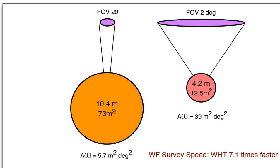
Figure 1: Survey efficiency of 10-m and 4-m telescopes compared. The speed at which one covers a given number of objects to a given S/N scales as the product of telescope collecting area  $A$  times viewing solid angle  $\omega$ . This product is  $5.7 \text{ m}^2 \text{ deg}^2$  for a 10-m telescope with a 20-arcmin FOV, and  $39 \text{ m}^2 \text{ deg}^2$  for a 4-m telescope with a 2-degree FOV. Survey speed is 7.1 times faster for the smaller telescope.
