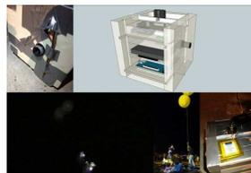
Launch images: (Bottom, left, center) D8 Draconids: two balloon configuration - D12-Geminids: (Up right) configuration diagram. (Up left) Watec 902H2 + Avenir 12mm F1.2. (Bottom right) Recovering stick. [LPI (2013) No. 1719, p.2202]
