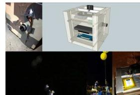
Launch images: (Bottom, left, center) D8 Draconids: two balloon configuration. D12-Geminids: (Up right) configuration diagram. (Up left) Watec 902H2 + Avenir 12mm F1.2. (Bottom right) Recovering stick. [LPI (2013) No. 1719, p.2202]
