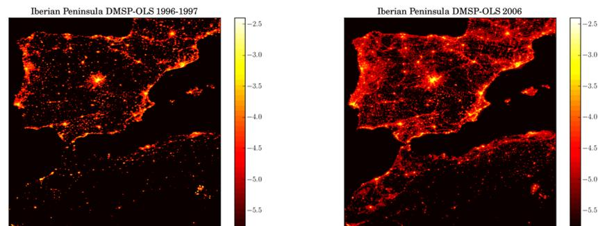
Evolution of the amount of light detected from space (1996-2006) with radiance calibrated data from DMSP-OLS satellite. The display scale is logarithmic and coded in units of W/m<sup>2</sup>/sr/um
