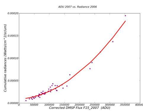
Coefficients to transform from RAW data (ADU) to radiance (W/cm<sup>2</sup>/sr/um) could be obtained for each satellite and date. The plot shows an example of the calibration of 2006 values to DMSP F15 (2007).
