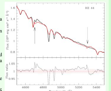
Top: Our spectrum (black) compared to CALSPEC tabulated spectrum (red) in the region where we found discrepancies (marked by arrows), most probably due to mismatch in CALSPEC spectrum (Bohlin, Dickinson, & Calzetti, 2001). Bottom: Ratio Ours/CALSPEC spectra and the ±1% margin of internal precision acceptance.
