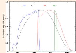
G, G<sub>BP</sub>, G<sub>RP</sub> and G<sub>RVS</sub> passbands corresponding to the measurement of white light, BP/RP and RVS fluxes
