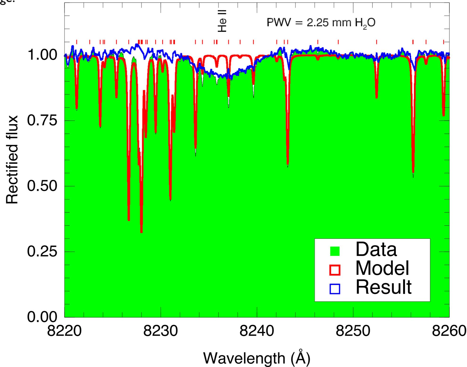
**Figure 5.** Elimination of H<sub>2</sub>O telluric lines in the H $\alpha$  region. Data obtained with HRS/HET at  $R = 30\,000$ . The red vertical bars mark the location of the strongest telluric lines in this wavelength range.
