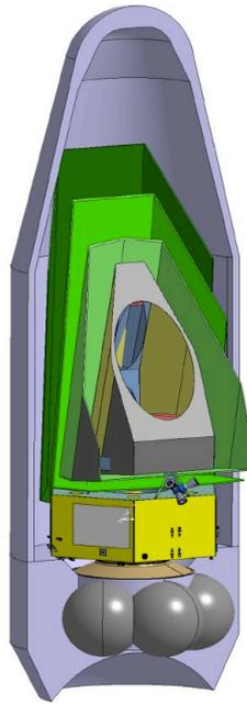
Figure 1: EChO modules and spacecraft design configurations under the Soyuz-Fregat fairing.
