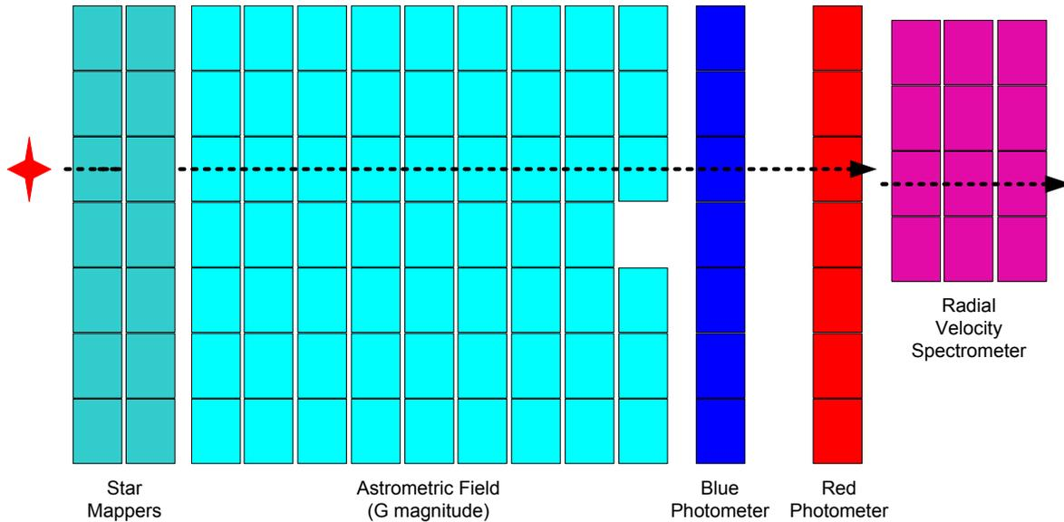
Figure 1: Gaia focal plane. Incoming images are detected by the star mapper, with separate CCDs for the two telescopes, while the rest of the focal plane is common.
