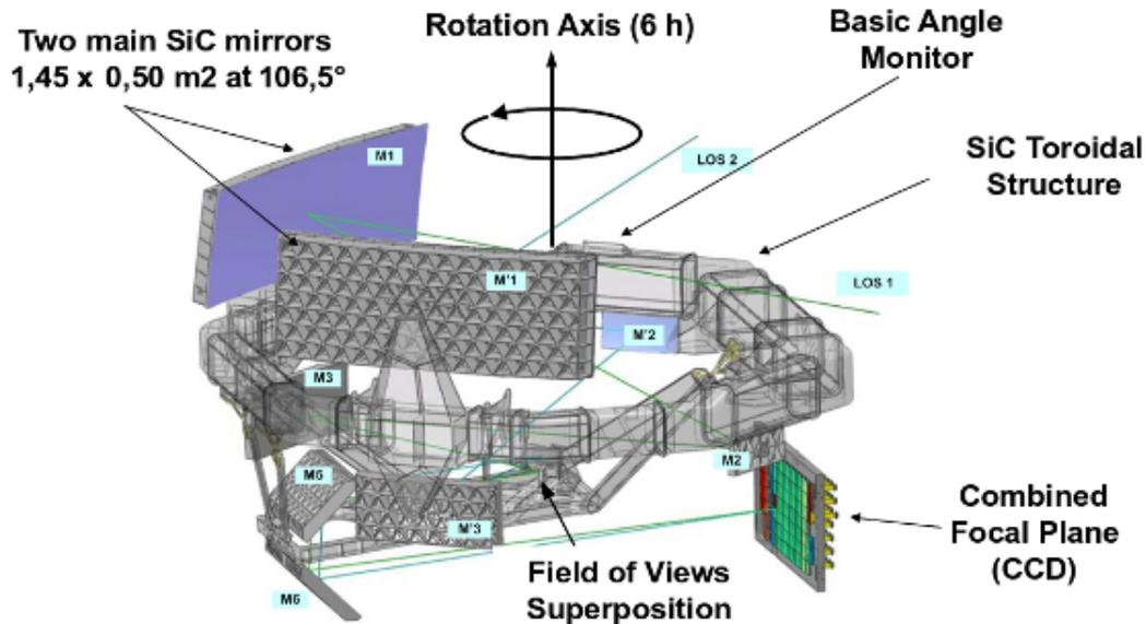
Figure 1: Gaia instrument combining two Lines Of Sight (LOS) at a single focal plane
