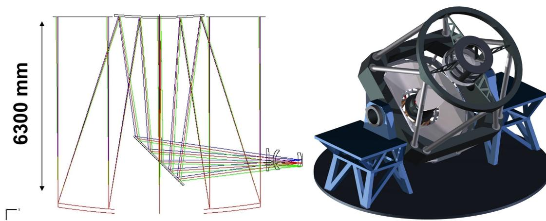
Figure 2: *Left panel:* Optical configuration for one of the HEXA design. In this case, a Ritchey-Chretien Nasmyth configuration with a  $1^\circ$  field-of-view. *Right panel:* 3D model for the telescope and the two Nasmyth platforms.
