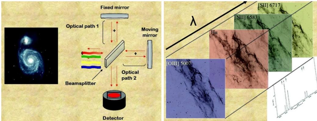
Figure 3: *Left panel:* Representation of a Michelson interferometer. *Right panel:* emission line maps resulting from an observation of a nebula with an IFTS.
