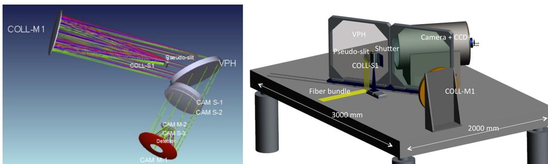
Figure 4: *Left panel:* 3D optical layout for GYGES, the medium-resolution multiobject spectrograph *Right panel:* 3D view on GYGES spectrograph of the optical bench.
