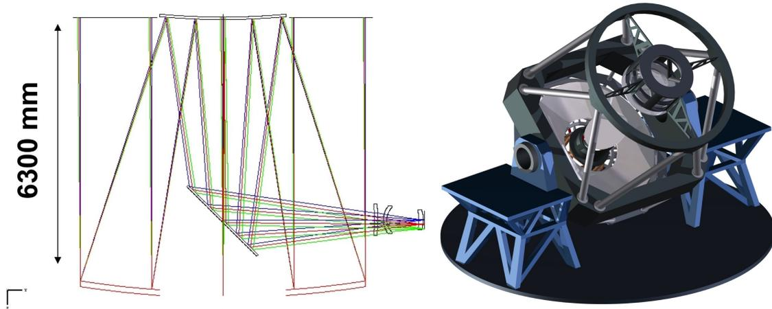
Figure 2: *Left panel:* Optical configuration for one of the HEXA design. In this case, a Ritchie Chretien Nasmyth configuration with a  $1^\circ$  field-of-view. *Right panel:* 3D model for the telescope and the two Nasmyth platforms.
