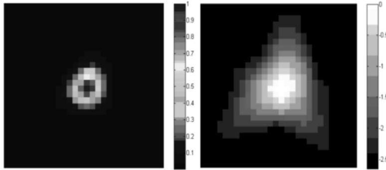
Figure 5: Simulation of the expected PSF for a point source (left) and in logarithmic scale (right).
