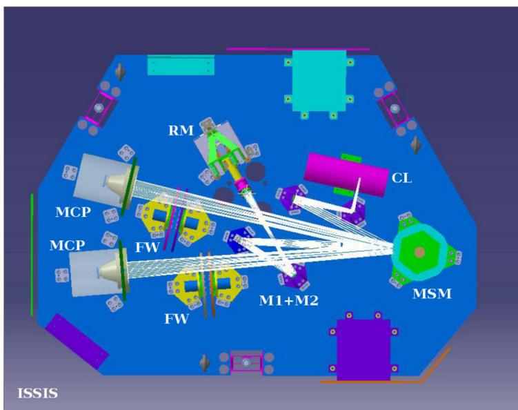
Figure 2: The optical bench assembly (without cover) for ISIS.
