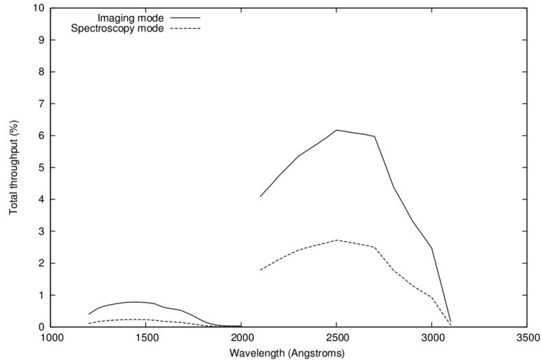
Figure 4: Throughput curves for the whole system in the two ISIS channels. The estimate includes the two telescope mirrors, the ISIS mirrors, the detector, and the grating (the latter one only in spectroscopy mode); filters are not considered.
