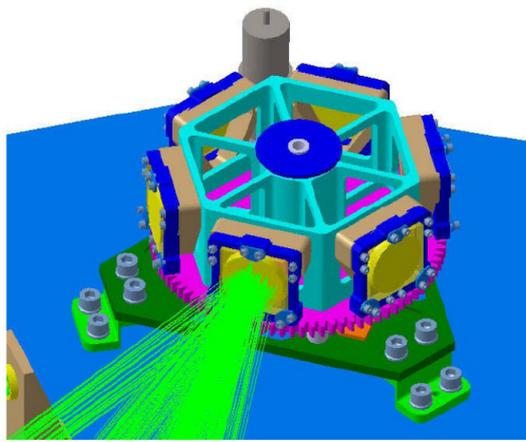
Figure 3: The mode selection mechanism (MSM) employed in ISIS.
