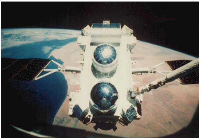
Figure 1.3: Left: Image of CGRO as it was being placed in orbit by Shuttle Atlantis. BATSE detectors can be seen at the corners of the satellite. Right: Diagram showing the structure of one of the BATSE detectors.
