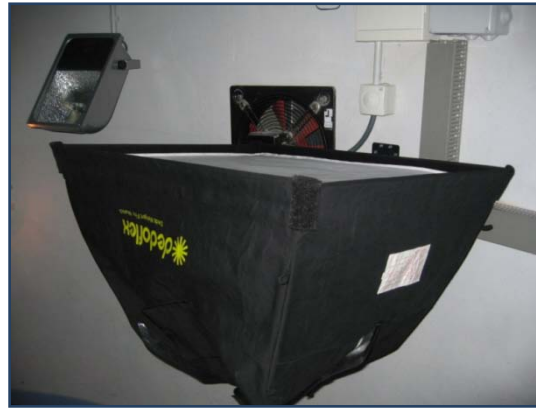
Fig. 4.17: Flat light mounted on the wall, with the diffuser surrounding the light
