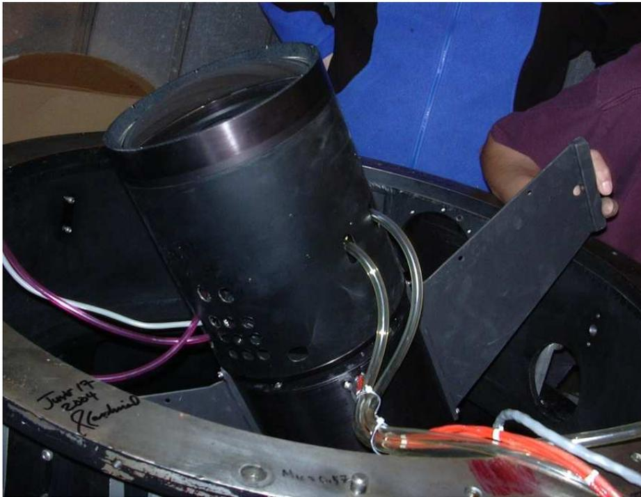
Figure A.11: Displaced spider vanes, focus and CCD housing of the NESS-T BNC while maintenance operations (courtesy of Rothney Astrophysical Observatory).
