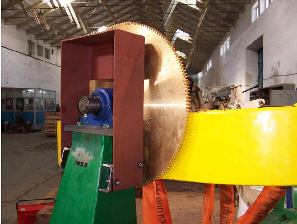
Figure A.10: Newly manufactured RA worm wheel drive installed at the RA axis.
