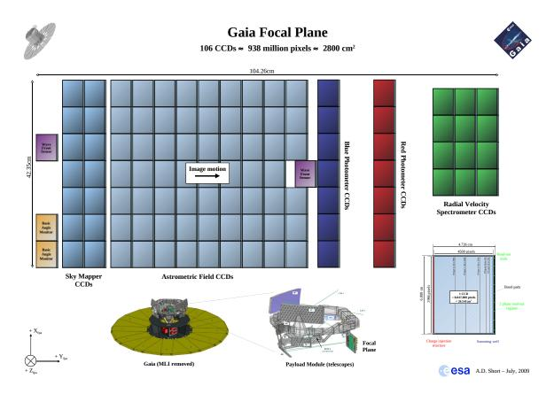
Figure 1: The Gaia focal plane. See text for details.
