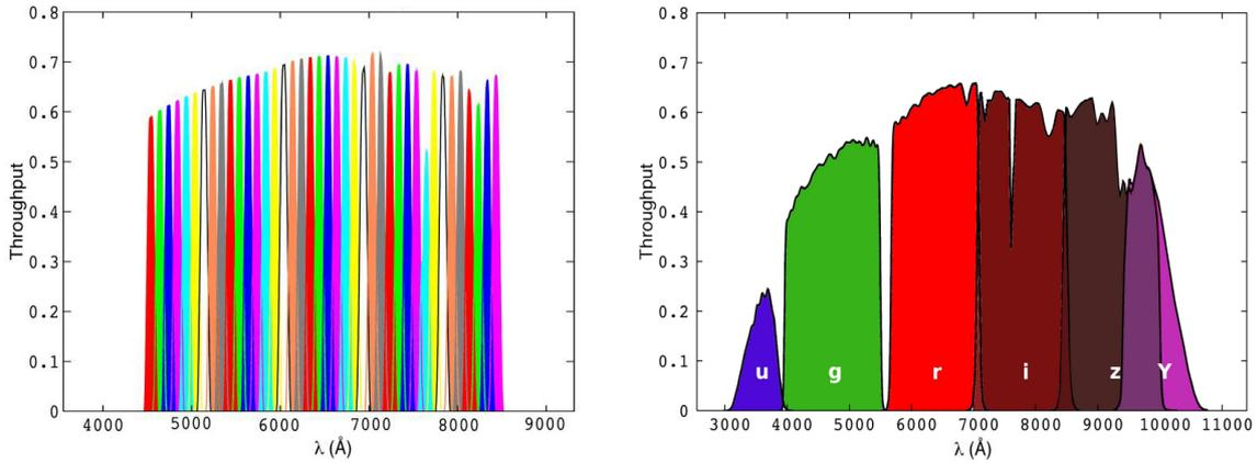
Figure 2: Theoretical throughput for the forty narrow-band filters (*left*) and for the six broad-band filters (*right*). These are calculated with models of the atmosphere, telescope and filter transmission and the quantum efficiency of HPKK detectors.
