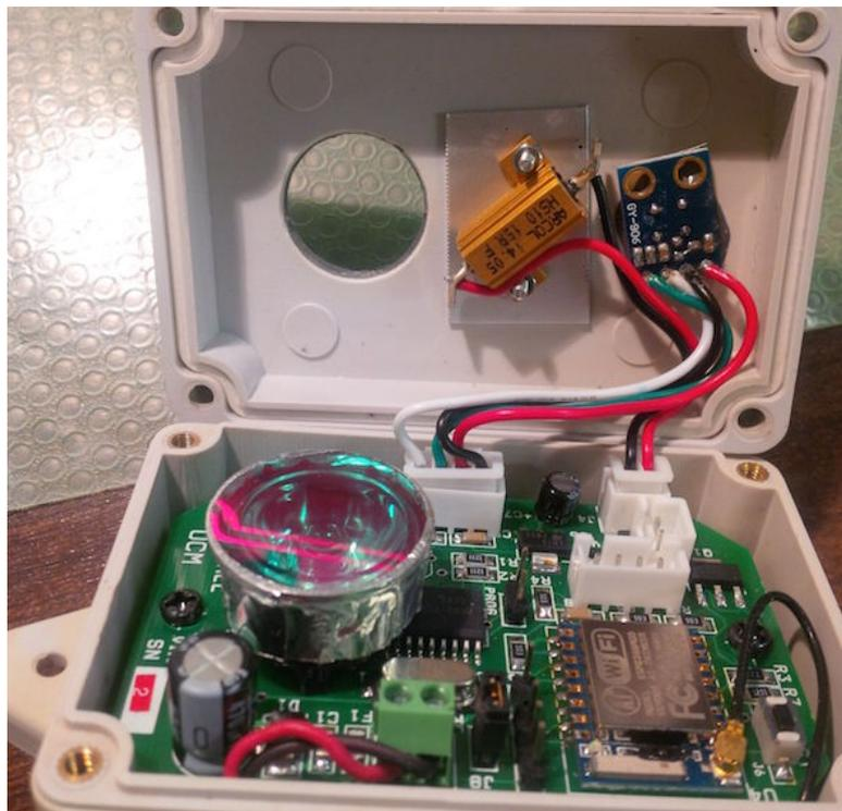
Figure 1: Internal view of the TESS-V1 night sky brightness photometer inside the weather proof box. The light collector with the infrared rejection filter (in blue) lies over the electronic PCBs.
