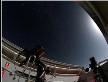
Fig 1. Inside the Monitor's building during a moonlight night. The telescope on the right is the current extinction monitor: EXCALIBUR while the one in the left is the DIMM, the seeing monitor.
