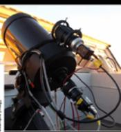
Fig 3. The seeing monitor. There are plans to move it to the top of a specific tower that will be built very soon to meet the standards of this type of observation, i.e. to measure a few meters below the ground level to get rid of the main contribution of the surface layer turbulence.
