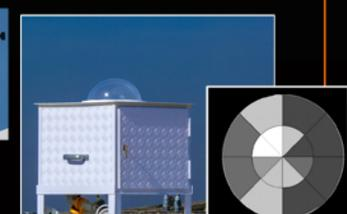
Fig 5. The ASTMON instrument (left picture) and a sample cloud coverage map (right diagram). This is the type of diagrams provided by ASTMON. The gray scale relies on the degree of cloud coverage: white areas means 100% covered while black ones indicates a cloud-free region (taken from Aceituno et al. 2011).
