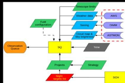
Fig 7: The Sequencer. This diagram shows the Sequencer's data flow (including the inputs coming from the Scheduler). The data provided by the Monitors and the AWS are encircled with a red dashed line. The output of the Sequencer is the final observation queue.
