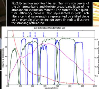
Fig 2. Extinction monitor filter set. Transmission curves of the six narrow-band and the four broad-band filters of the atmospheric extinction monitor. The current CCD's quantum efficiency curve is also represented in pink. Each filter's central wavelength is represented by a filled circle on an example of an extinction curve (in red) to illustrate the sampling of this curve.
