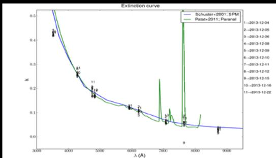
Fig 6: Results from a sample of nights. The numbers are placed on the obtained extinction coefficients from the extinction monitor data during the indicated nights. These values are compared to published extinction curves (top panel) from Paranal (Patat et al. 2011) and San Pedro Mártir (Schuster et al. 2001); the later from spectroscopic data. The fitted coefficients and their dispersions are shown in
