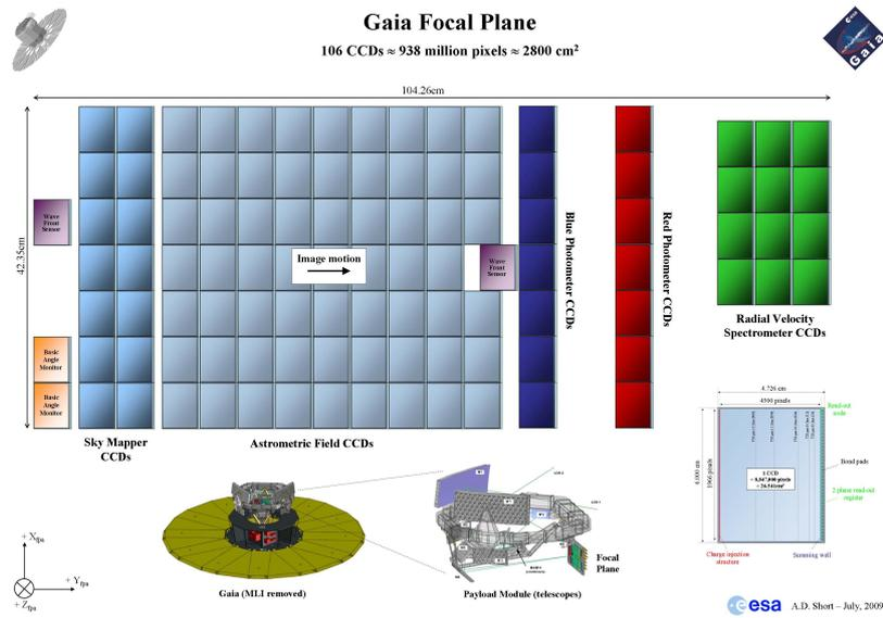
Figure 6: The Gaia focal plane. The images of the two viewing directions are superimposed on it.
