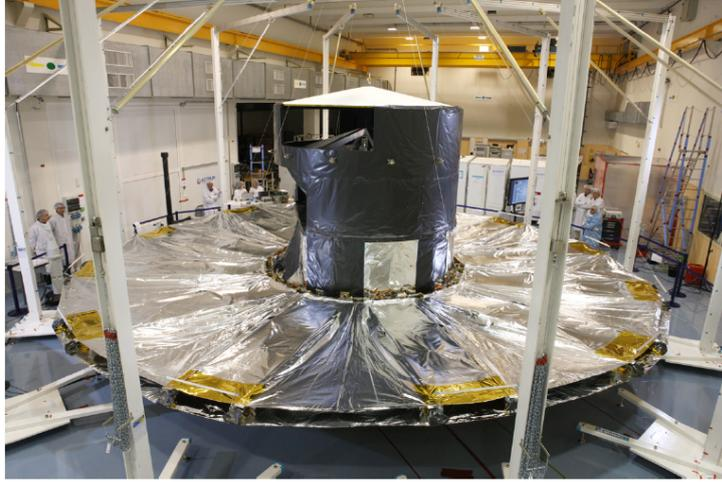
Figure 1: The Gaia satellite after a sunshield deployment test (image courtesy EADS-Astrium).
