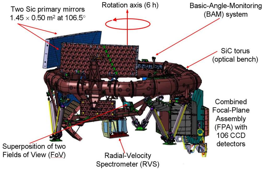
Figure 5: The payload core is a SiC torus supporting all the optical elements and the focal plane assembly
