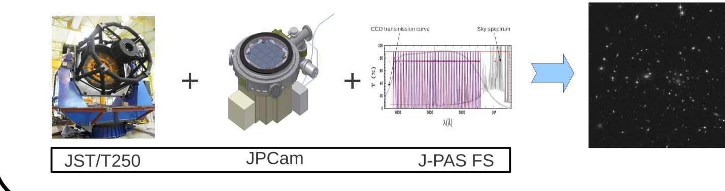
Secondary standard stars are identified in each CCD of the JPCam. Comparison between observed magnitudes and synthetic ones will produce the photometric zero points to be used with all the objects in the same exposure.
